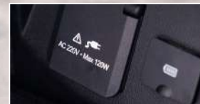
120 WATT 220V INTERIOR POWER OUTLET.
